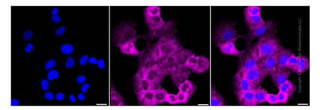
Immunocytochemical staining of HT-1080 cells with anti-Opioid receptor delta 1 antibody (Cat#2317, 1:1,000). Nuclei were stained blue with DAPI; Opioid receptor delta 1 was stained magenta with Alexa Fluor® 647. Images were taken using Leica stellaris 5. Protein abundance based on laser Intensity and smart gain: Medium. Scale bar: 20 µm.
