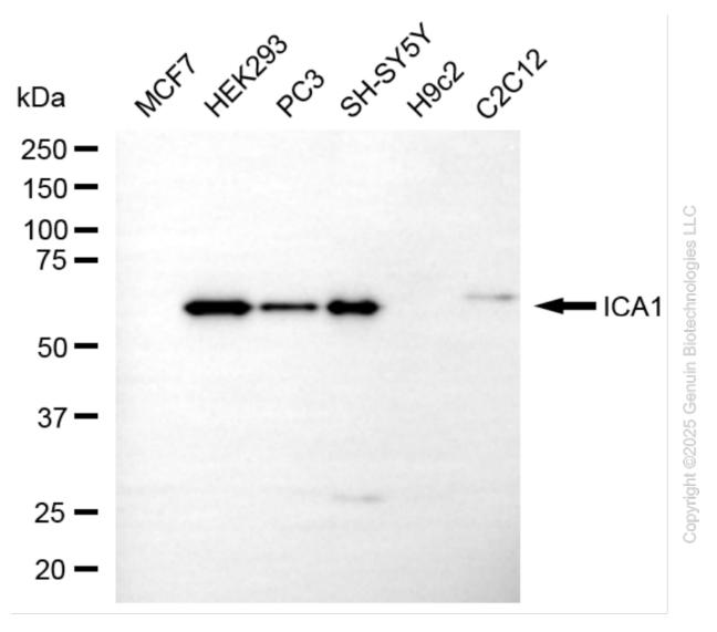
Western blotting analysis using anti-ICA1 antibody (Cat#5287). Total cell lysates (30 μg) from various cell lines were loaded and separated by SDS-PAGE. The blot was incubated with anti-ICA1 antibody (Cat#5287, 1:2,000) and HRP-conjugated goat anti-mouse secondary antibody (Cat#101, 1:20,000) respectively. Image was developed using FeQ<sup>TM</sup> ECL Substrate Kit (Cat#226).
