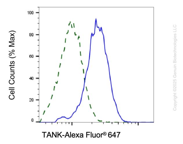
Validation of TANK knockdown using flow cytometry. Wild-type(WT, Blue) and knockdown(KD, Green) HeLa cells were stained with anti-TANK antibody (Cat#65874, 1:2,000) and analyzed using BD flow cytometer.
