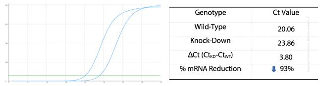
RT-qPCR analysis. HeLa cells were infected with NUP155-specific shRNA lentiviral particles, total RNA was extracted from wild-type and knockdown cells, RT-qPCR was performed using gene-specific primers.  $\Delta$ Ct (CtKD-CtWT) was used to calculate mRNA reduction (%) between wild-type and knockdown cells using the following formula:  $(1-1/2\Delta$ Ct) x 100%.
